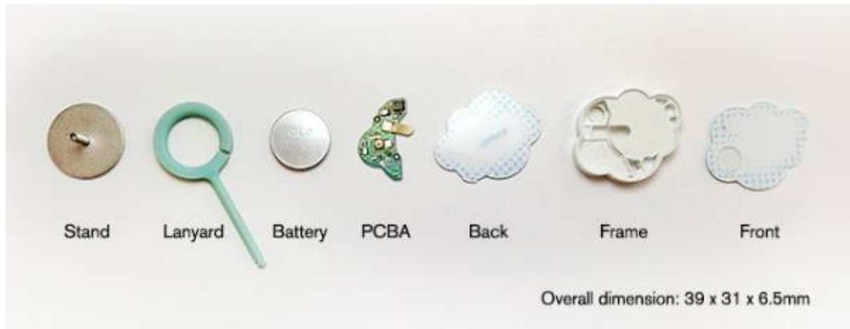
Figure 8: Parts and size of the CliMate [(kickstarter)]
