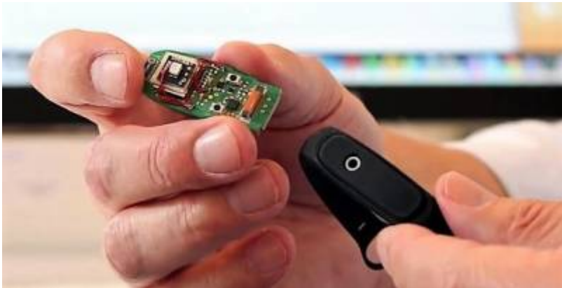
Figure 6: Electrical components inside the Raymio
