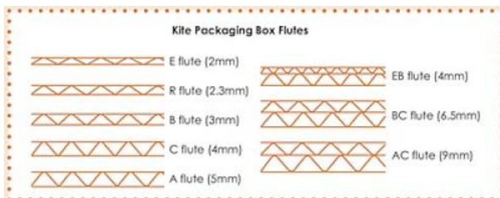
Figure 43: Corrugated Cardboard types [(corrugated)]
