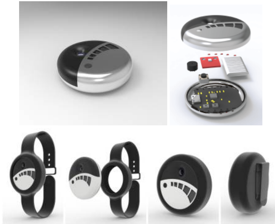
Figure 29: Improved 3D model with bracelet and clip-on
