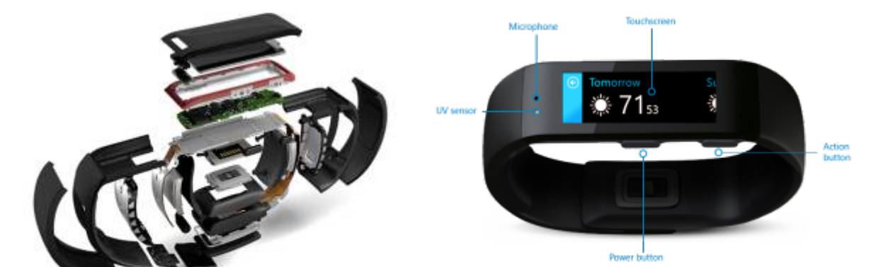
Figure 4: Components and UV sensor position of the Microsoft Band [(microso)]
